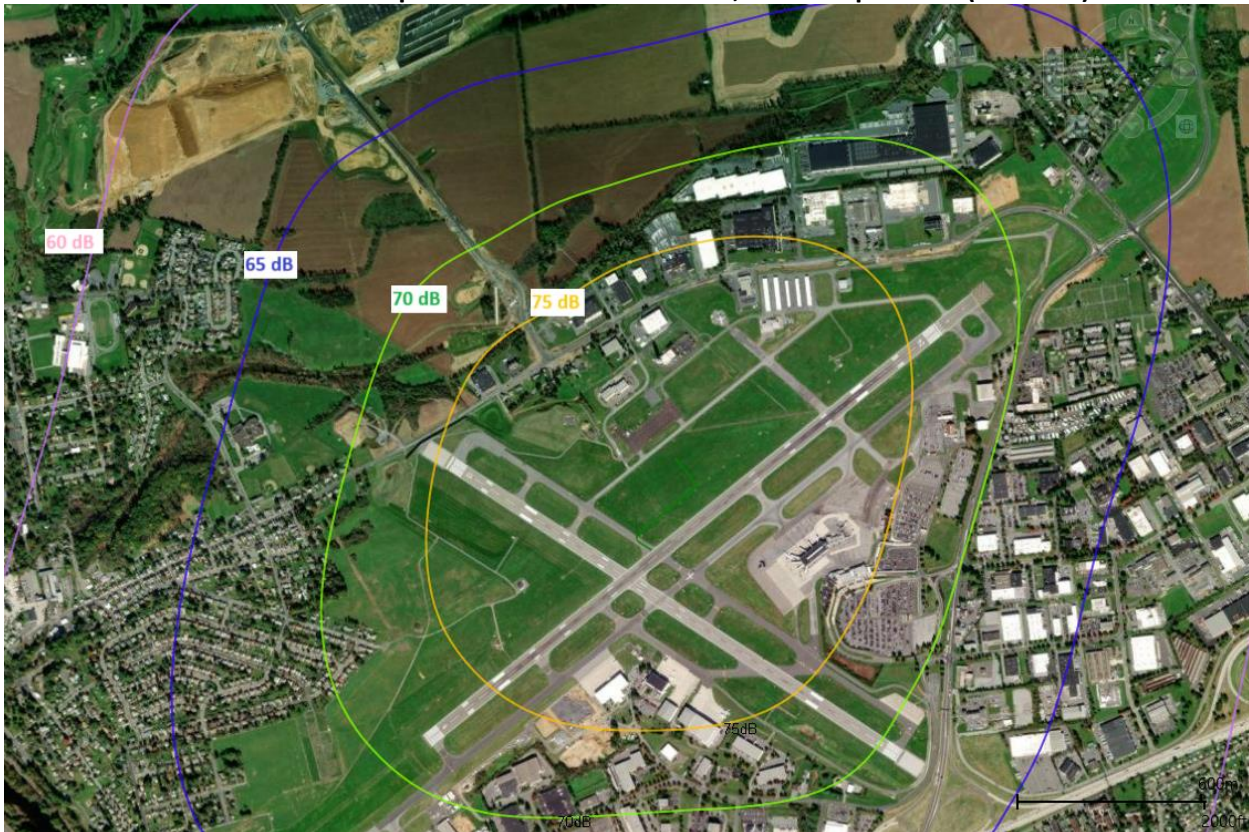
Figure 8 B767-300 Sound Exposure Level Noise Contour, Arrival Operation (B-D-NCA)
