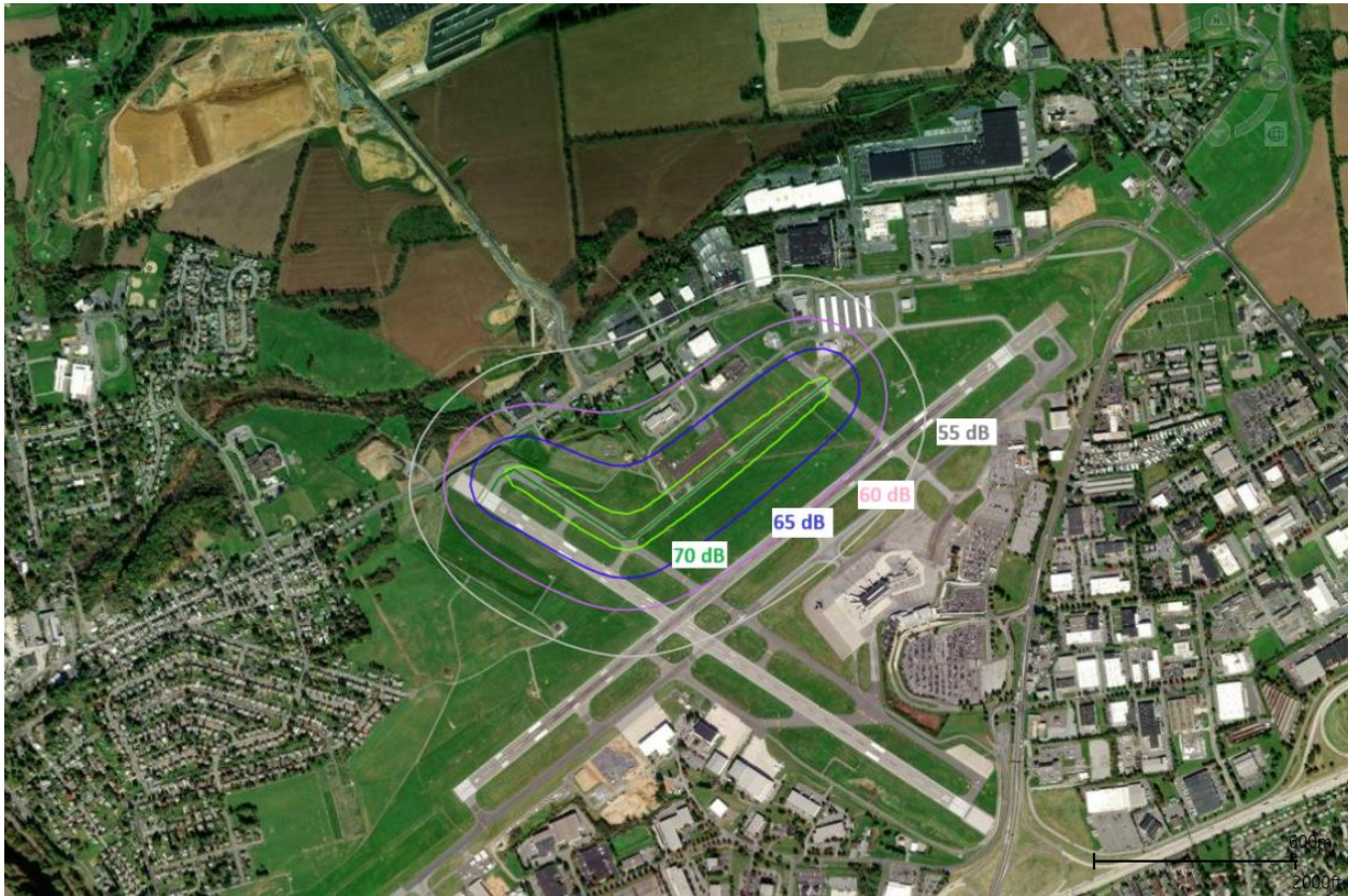
Figure 5 PA-28 Sound Exposure Level Noise Contour, Departure Operation (Hangar 5-C-B-B7)
