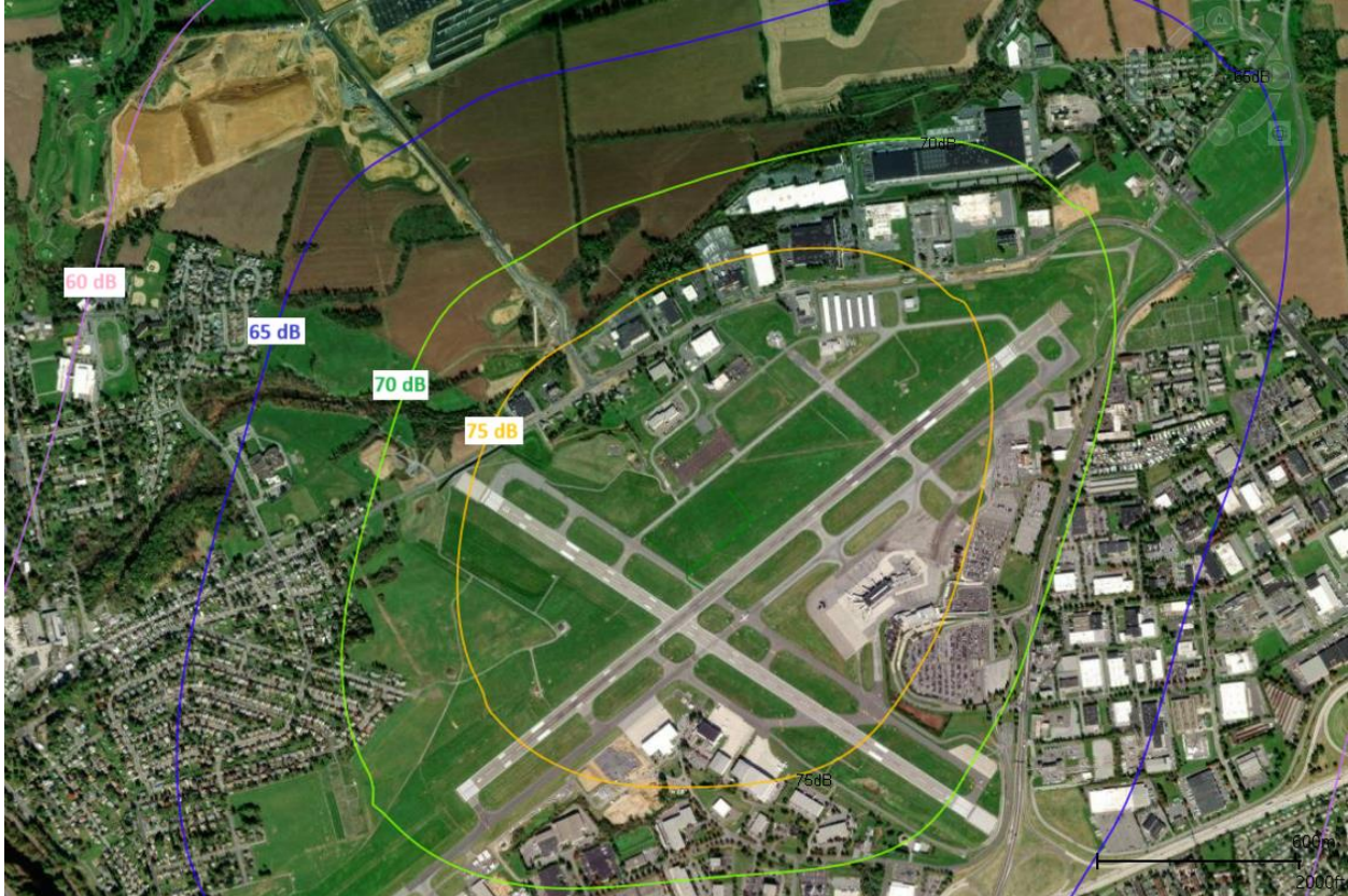
Figure 7 B767-300 Sound Exposure Level Noise Contour, Departure Operation (NCA-D-B)
